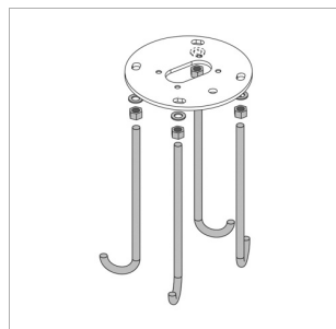
Anchor Bolts w/ template Ø0.64" x 17" long 3" hook Top 3.25" threaded
